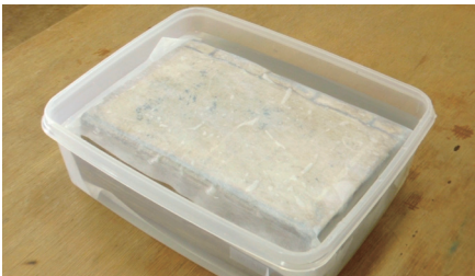
4. 次亜塩素酸ナトリウム水溶液（400ppm）による殺菌洗浄 4. Cleaning and sterilization using a sodium hypochlorite aqueous solution with a concentration of 400 ppm
